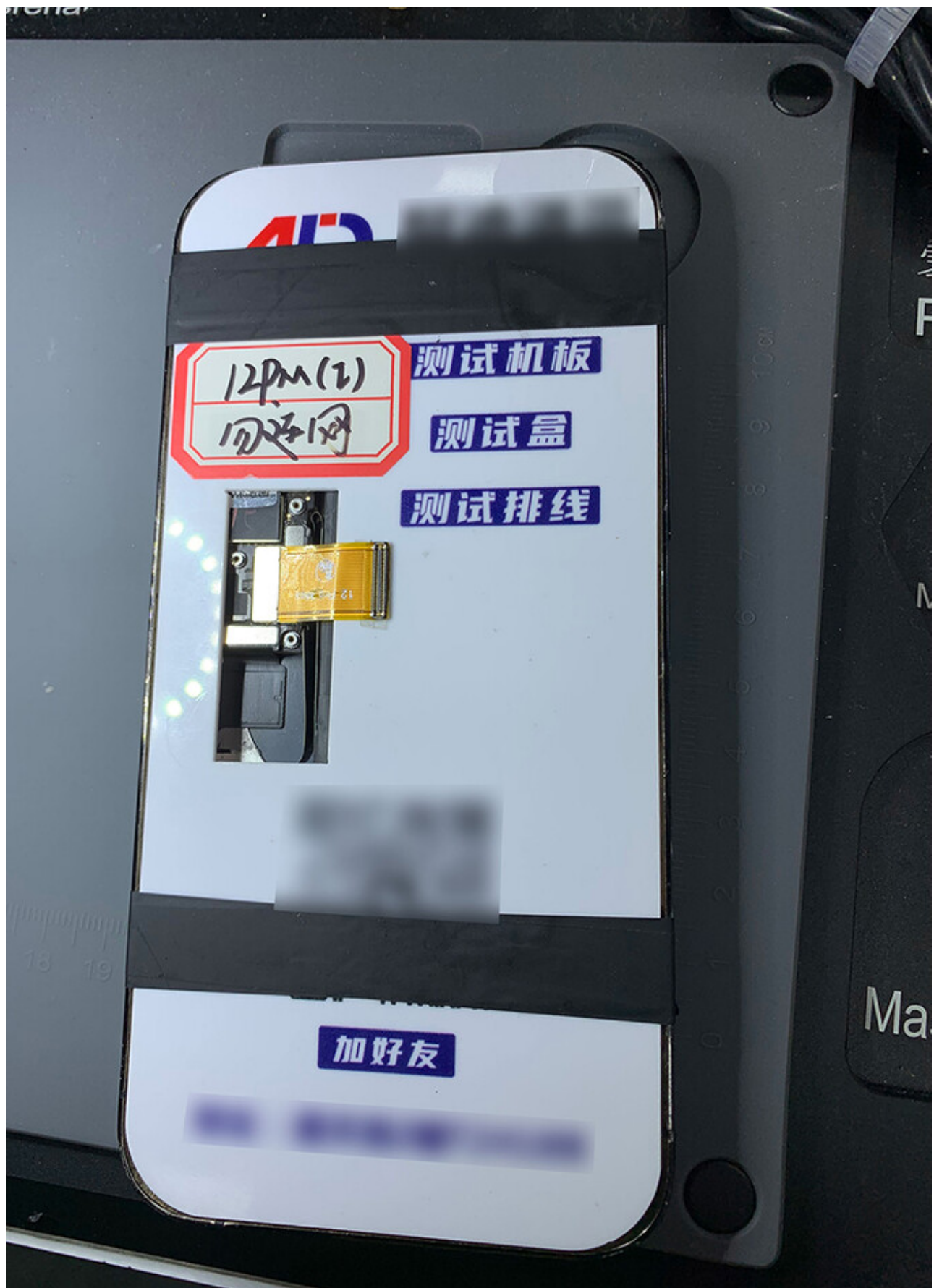
A self-made diagnostic tool to test screen functionality, repurposed from a display-less smartphone, 2024. Photo: Yifan Wang.
