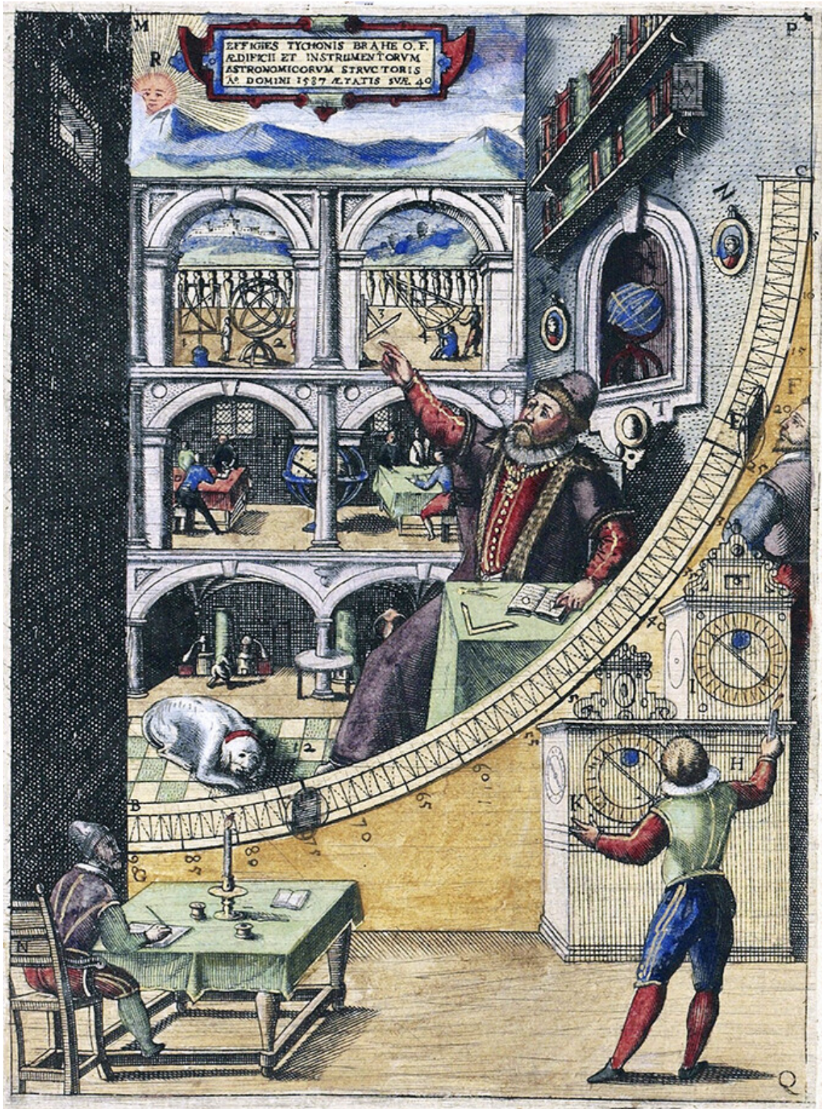
Tycho Brahe's mural quadrant in Uraniborg (Uraniborg). The quadrant (radius c. 194 cm) was made from brass and was affixed to a wall that was oriented precisely north-south. The observer (far right) views a star through the opposite opening (upper left) to determine the star's altitude as it passes through the meridian. An assistant (lower right) reads the time off a clock and another one (lower left) records the measurements. The area above the quadrant is filled with a mural painting showing several other of Brahe's instruments. License: Public domain.
