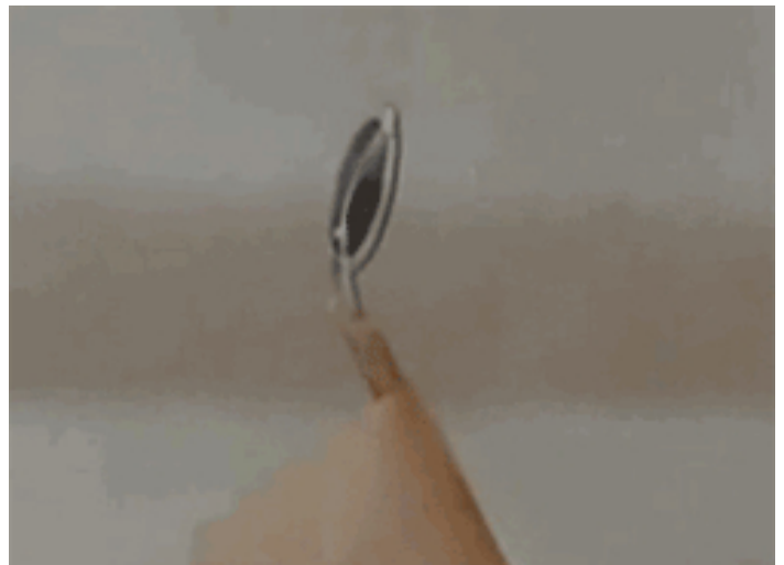
Prototype of LCD screen in a curved contact lens by a team of researchers at Ghent University. To demonstrate the capacity to form simple images on the conductive polymers of the lens scientists chose a flashing dollar sign.
